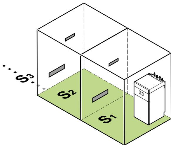
$$S_1 + S_2 + S_3 + \dots \geq S(m^2)$$
